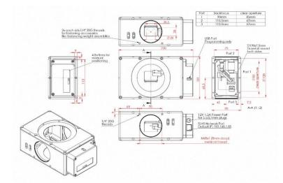
The IMP85 has **a unique** selling point with its **unmirrored port**1. Where other devices have a central mirror that rotates, the design of the IMP85 keeps the main camera in the central focus. No light is lost and the weight is evenly distributed. The compact and massive construction enables the shortest possible connection to many telescope systems.
